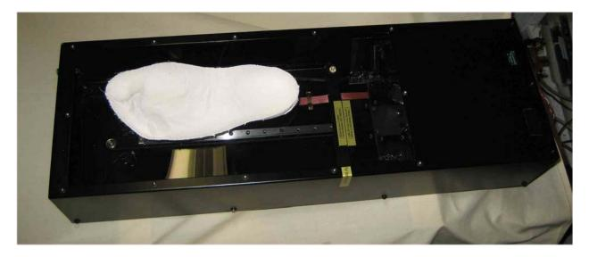
The bottom of the cast can be treated with black dots on 1<sup>st</sup> and 5<sup>th</sup> met. heads and the foot can be balanced on the scanner with a wedge as shown below.
